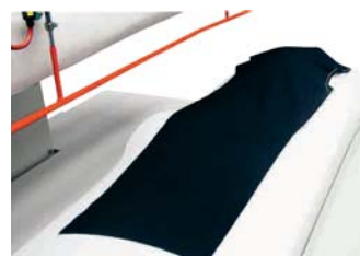
Cylinder for shaping effect in the waist area of back center seam
